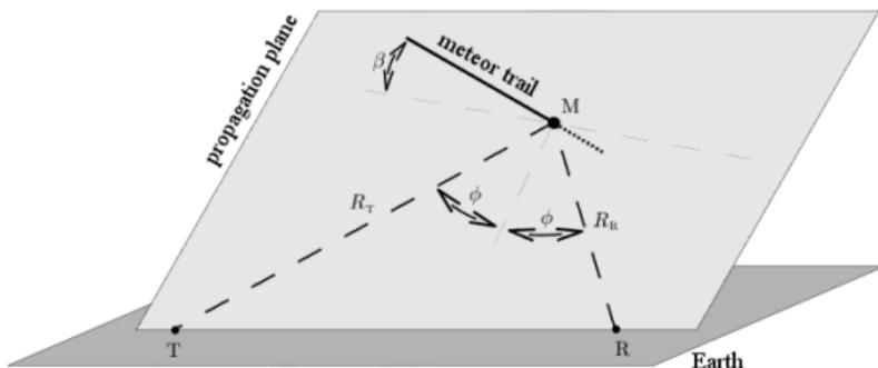
The geometry of this situation includes the influence of **half forward-scatter angle** ( $\phi$ ) on the received signal level...
